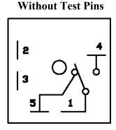
The agitation timer is standard equipment for the floor standing dispenser. The purpose of the timer is to periodically agitate the ice in the bin to prevent congealing. Non adjustable timers with test pins are used on all current production models.
